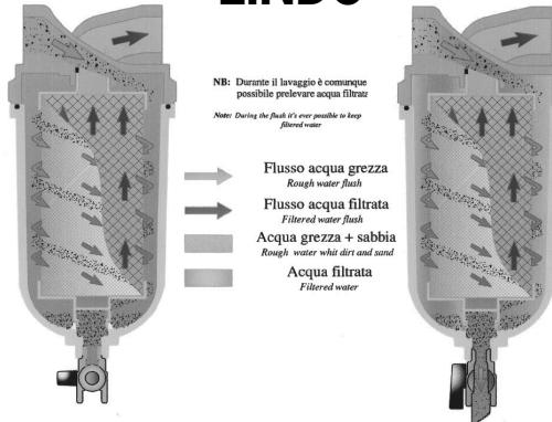
They are endowed with a stainless steel cartridge, chromium-plated brass head and ring. They can be easily cleaned by operating the exhaust-valve on the bottom.
